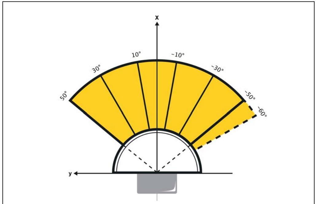
Fig. 3-15: Scanning frequency 50 Hz with constant angular resolution of 0.5°
