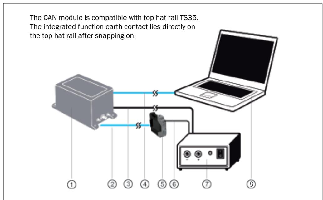
Fig. 5-2: Field monitoring: Electrical installation of the LD-MRS and the CAN module
