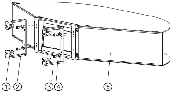
Version 2: Install the bracket by introducing the screws from the front
