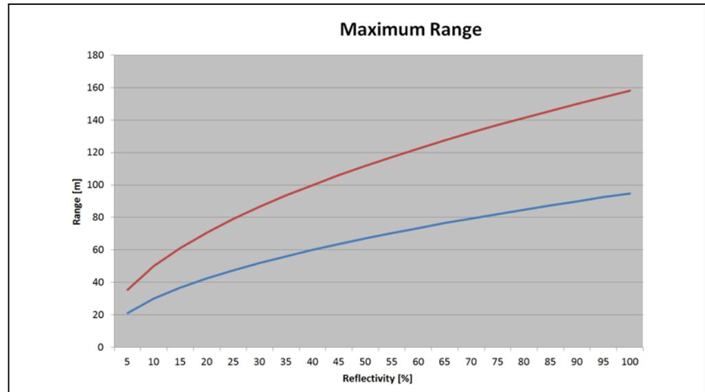
Fig. 3-8: Sensing range in relation to remission
