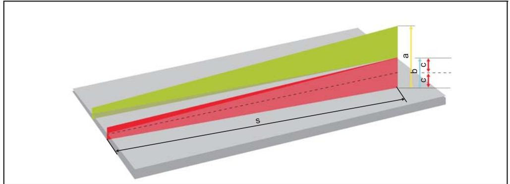
Fig. 4-1: Beam expansion
