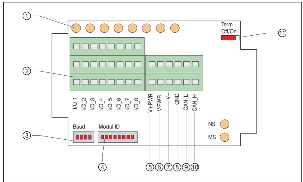
Fig. 5-4: Design of the CAN module  $\mu$ CAN.8.dio-BOX
