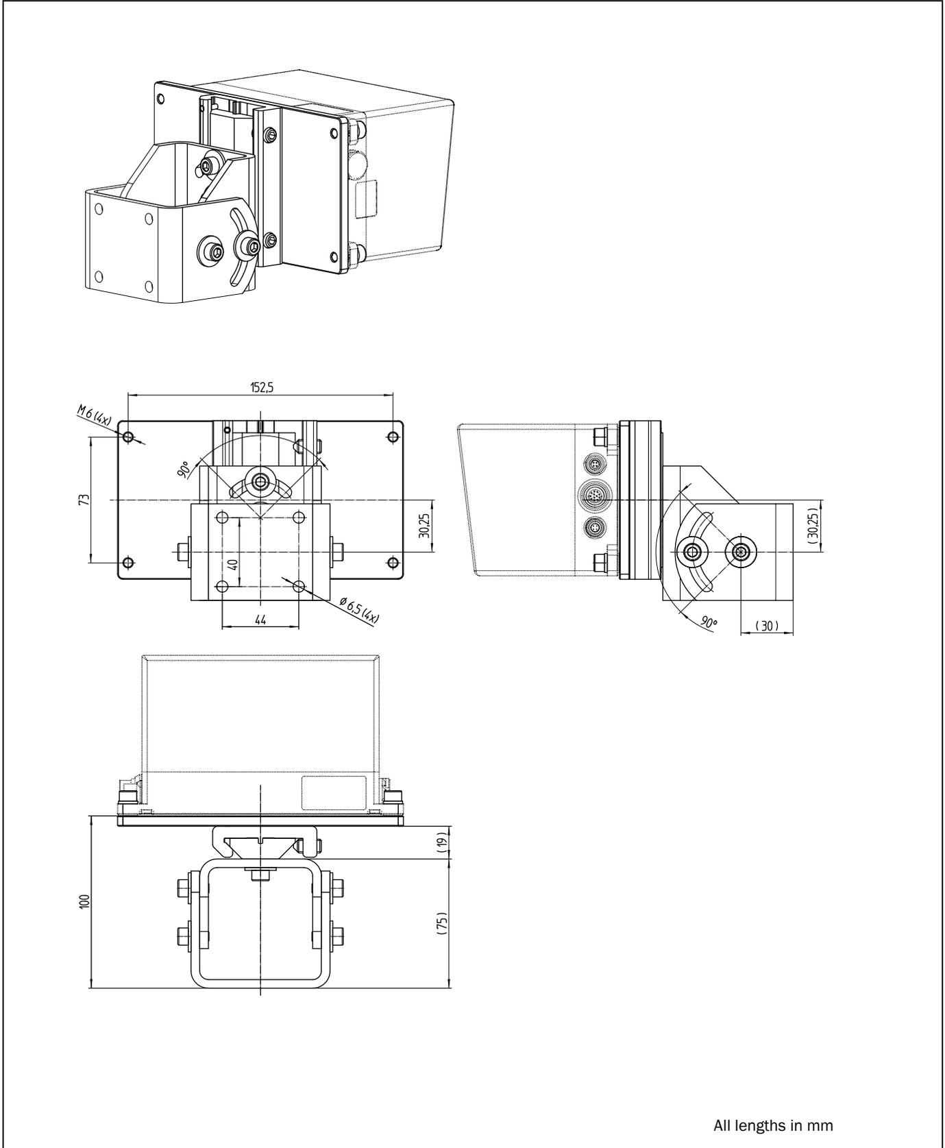
Fig. 9-4: Dimensions of the holder Part No. 1047429
