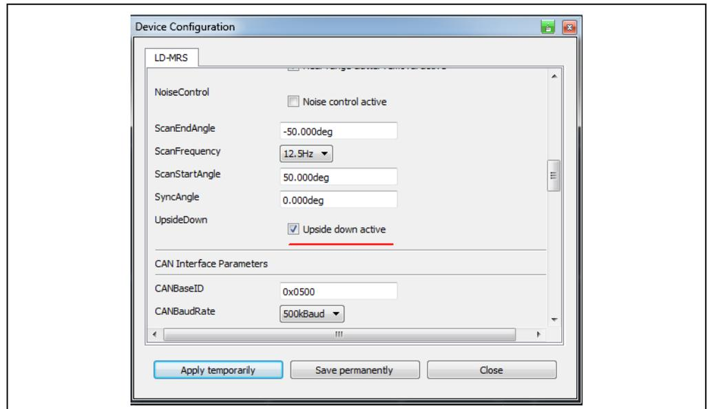
Fig. 3-29: Device parameter: Upside down mounting
