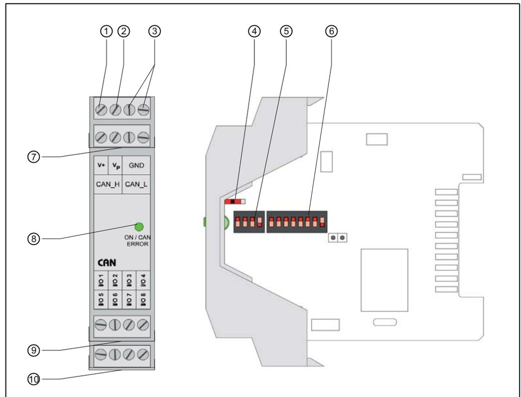
Fig. 5-5: Design of the CAN module  $\mu$ CAN.8.dio-SNAP
