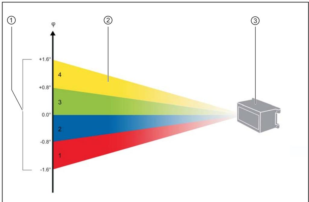
Fig. 3-5: Principle of the scan planes, color-coded
