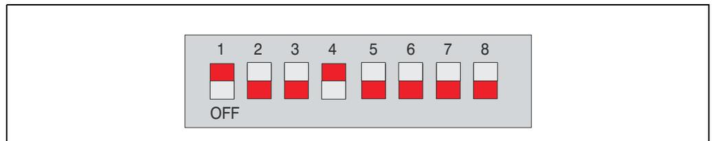
Fig. 5-10: DIP switch for address (example: address 9)
