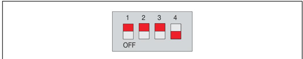
Fig. 5-11: DIP switch for transmission rate (example: 500 kBit/s)
