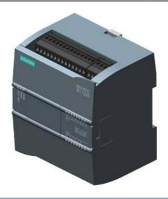
SIMATIC S7-1200, CPU 1212C, COMPACT CPU, DC/DC/RLY, ONBOARD I/O: 8 DI 24V DC; 6 DO RELAY 2A; 2 AI 0 - 10V DC, POWER SUPPLY: DC 20.4 - 28.8 V DC, PROGRAM/DATA MEMORY: 50 KB
