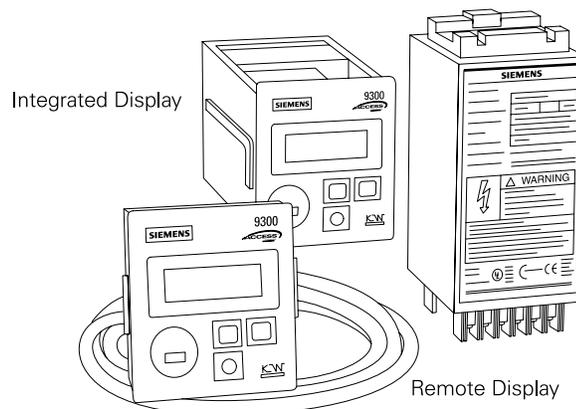
The 9300 includes a front optical data port for accessibility by a portable PC.
