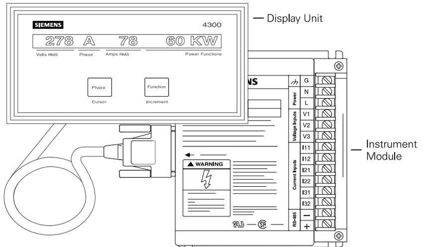
The 4300 meter is designed to fit in new or retrofit applications. The display unit will fit standard U.S. analog meter drilling patterns.
