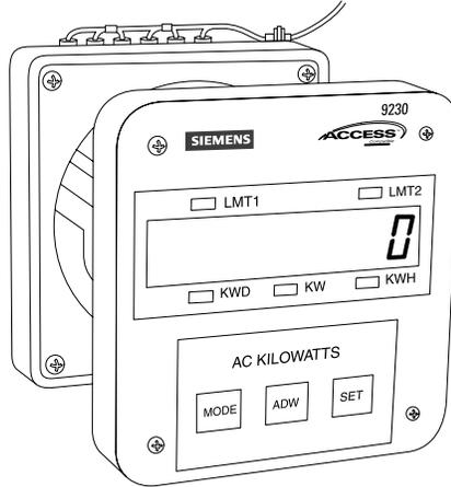
The 9230 meter measures voltage and current to calculate power. Alarm functions can be programmed to operate two relay contacts. A KYZ relay provides pulses for energy management systems. These pulses represent accumulated positive or negative watt-hours. The pulse value is configurable. SEABus communication converters or analog output modules are available.
