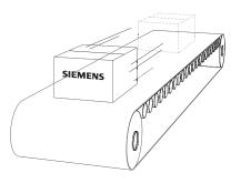
Work is generally expressed in foot-pounds and is defined by the product of the net force (F) applied and the distance (d) moved. If twice the force is applied, twice the work is done. If an object moves twice the distance, twice the work is done.
