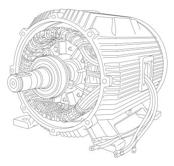
The enclosure also protects the electrical and operating parts of the motor from harmful effects of the environment in which the motor operates. Bearings, mounted on the shaft, support the rotor and allow it to turn. A fan, also mounted on the shaft, is used on the motor shown below for cooling.
