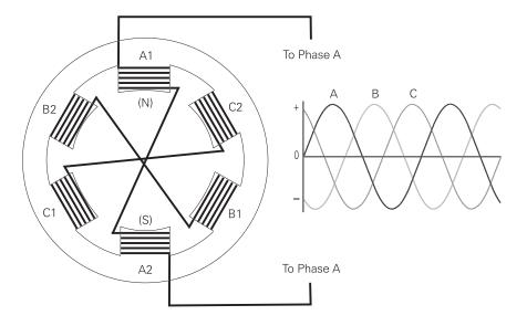
Phase windings (A, B, and C) are placed 120° apart. In this example, a second set of three-phase windings is installed. The number of poles is determined by how many times a phase winding appears. In this example, each phase winding appears two times. This is a two-pole stator. If each phase winding appeared four times it would be a four-pole stator.
