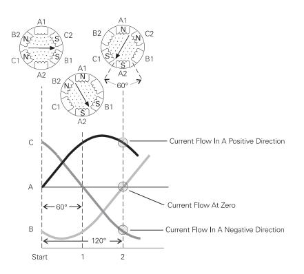
At the end of six such time intervals the magnetic field will have rotated one full revolution or 360°. This process will repeat 60 times a second on a 60 Hz power supply.
