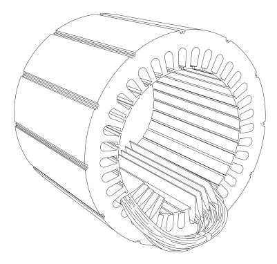
Each grouping of coils, together with the steel core it surrounds, form an electromagnet. Electromagnetism is the principle behind motor operation. The stator windings are connected directly to the power source.
