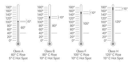
The operating temperature of a motor is important to efficient operation and long life. Operating a motor above the limits of the insulation class reduces the motor's life expectancy. A 10° C increase in the operating temperature can decrease the motor's insulation life expectancy as much as 50%. **Motor Design**
