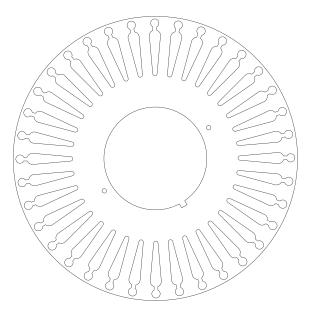
The laminations are stacked together to form a rotor core. Aluminum is die cast in the slots of the rotor core to form a series of conductors around the perimeter of the rotor. The conductor bars are mechanically and electrically connected with end rings. The rotor core mounts on a steel shaft to form a rotor assembly.
