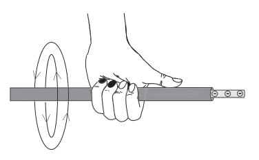
In the following illustration it can be seen that when the electron flow is away from the viewer (indicated by the plus sign) the lines of flux flow in a counterclockwise direction around the conductor. When the electron flow reverses and current flow is towards the viewer (indicated by the dot) the lines of flux reverse direction and flow in a clockwise direction.
