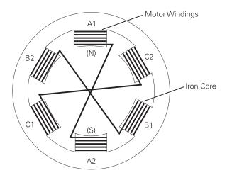
The stator is connected to a 3-phase AC power supply. In the following illustration phase A is connected to phase A of the power supply. Phase B and C would also be connected to phases B and C of the power supply respectively.
