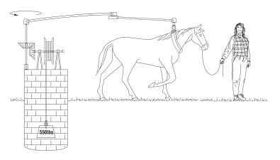
The following formula can be used to calculate horsepower when torque (in lb-feet) and speed are known. An increase of torque, speed, or both will cause an increase in horsepower.
