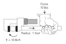
An increase in force or radius would result in a corresponding increase in torque. Increasing the radius to two feet, for example, results in 20 lb-ft of torque.
