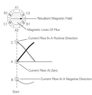
If the field is evaluated at 60° intervals from the starting point, at Time 1, it can be seen that the field will rotate 60°. At Time 1 phase C has no current flow, phase A has current flow in a positive direction and phase B has current flow in a negative direction. Following the same logic as used for the starting point, windings A1 and B2 are north poles and windings A2 and B1 are south poles.
