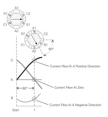
At Time 2 the magnetic field has rotated 60°. Phase B has no current flow. Although current is decreasing in phase A it is still flowing in a positive direction. Phase C is now flowing in a negative direction. At start it was flowing in a positive direction. Current flow has changed directions in the phase C windings and the magnetic poles have reversed polarity.
