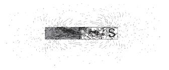
By drawing lines the way the iron filings have arranged themselves, the following illustration is obtained. Magnetic lines of flux always form closed loops, leaving the north pole and entering the south pole. They return to the north pole through the magnet.
