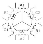
2-Pole Stator Winding
