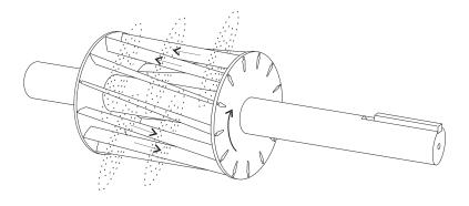
The following drawing illustrates one instant in time during which current flow through winding A1 produces a north pole. The expanding field cuts across an adjacent rotor bar, inducing a voltage. The resultant magnetic field in the rotor tooth produces a south pole. As the stator magnetic field rotates the rotor follows.
