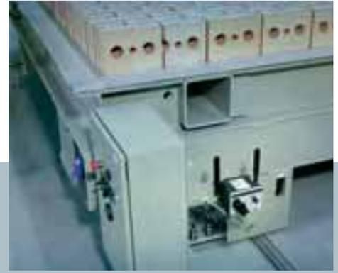
PROFINET I/O Controllers, SCALANCE W access points and client modules, as well as the IWLAN PB PN IO Link, were integrated into the PROFINET communication system.
