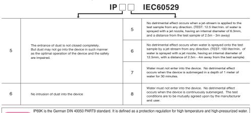
1P69K is the German DIN 40050 PART9 standard. It is defined as a protection regulation for high temperature and high-pressurized water.
