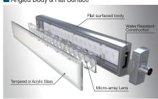
The side body angle was designed to prevent dirt accumulation. and for water and oil to roll off the surface. The LED lens retains a simple flat-surface for lighting and to help when wiping it down.
