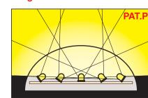
Patlite has created a revolutionary lighting design (patent pending) in which multiple LEDs project light across a broad peripheral area, ensuring equal intensity at the sides as well as the front. This design, with its side-projection technology, is a unique achievement in signal light
