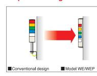
Patlite has perfected a 37.5mm-thin design that significantly enhances integration with the equipment as a built-in signal system.
