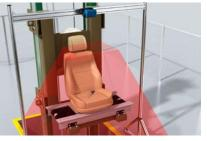
Detection of undesirable deviations by comparing an image against a predefined model to recognize improper conditions. In the image on the right, there is a screwdriver on the seat.
