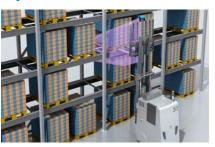
Precise position detection of a pallet for loading or unloading tasks in a high-bay warehouse.
