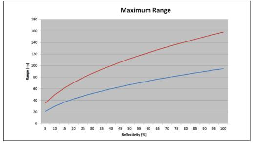
Fig. 3-8: Sensing range in relation to remission
