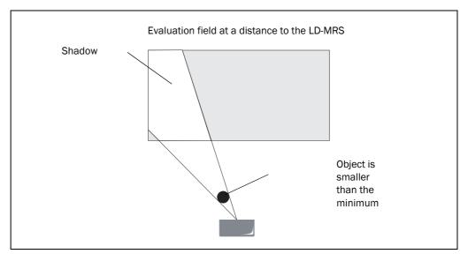
Fig. 3-31: Manipulation protection against shadow
