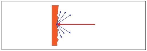
Fig. 3-16: Reflection of the laser beam at the surface of an object
