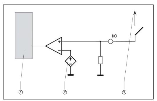
Fig. 5-8: Input switched against V<sub>+PWR</sub>
