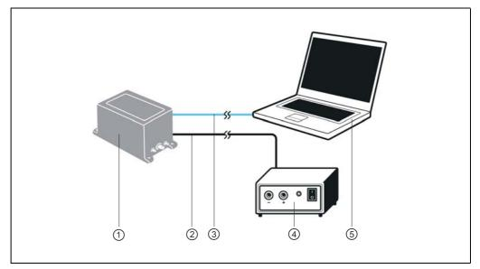
Fig. 5-1: Measuring mode: Electrical installation of the LD-MRS
