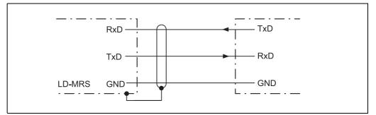
Fig. 5-12: Wiring of the RS-232 interface
