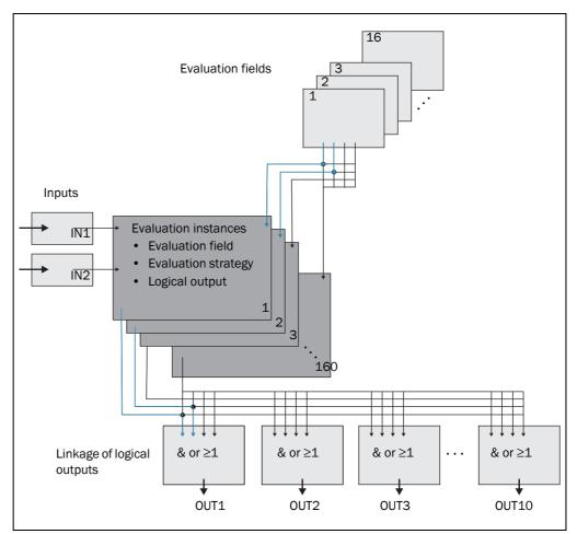
Fig. 3-30: Principle of field monitoring
