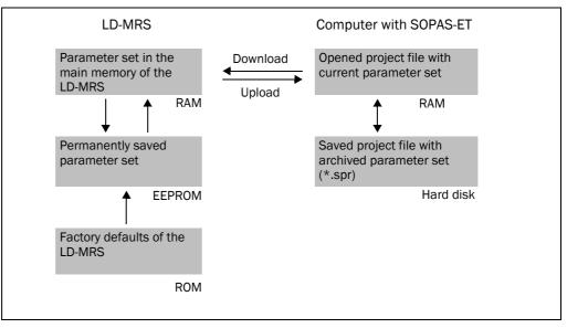
Fig. 6-1: Principle of data storage
