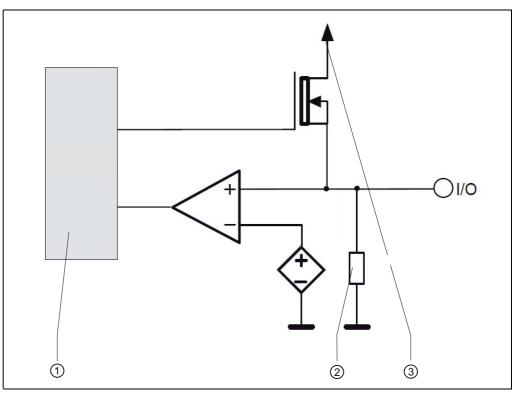
Fig. 5-9: A circuit diagram of digital I/O terminal (high side driver)
