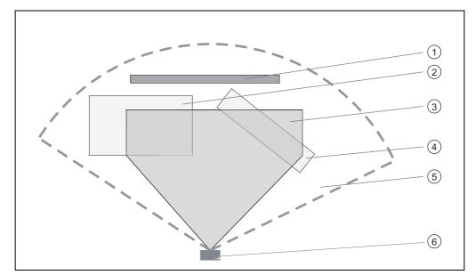
Fig. 3-32: Examples of evaluation field shapes
