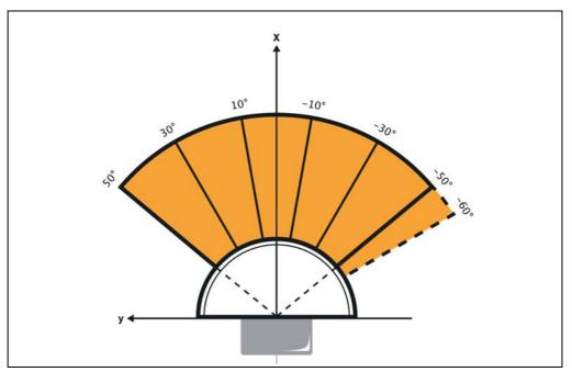
Fig. 3-13: Scanning frequency 12.5 Hz with constant angular resolution of 0.25°
