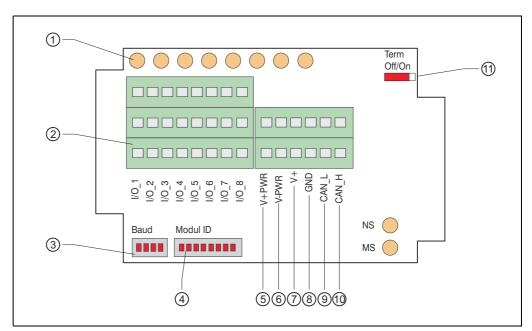
Fig. 5-4: Design of the CAN module µCAN.8.dio-BOX
