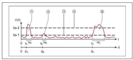
Fig. 3-9: Example of three echoes of a laser pulse
