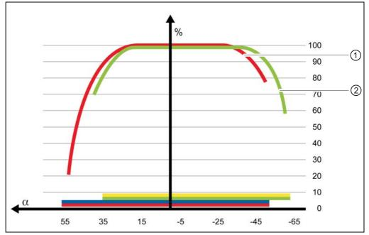
Fig. 3-7: Relation of angle to scanning range
