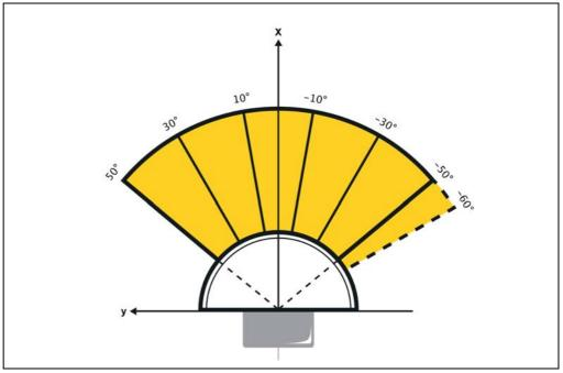
Fig. 3-15: Scanning frequency 50 Hz with constant angular resolution of 0.5  $^\circ$
