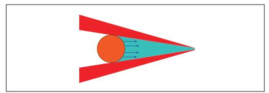
Fig. 3-20: Object smaller than diameter of the laser beam
