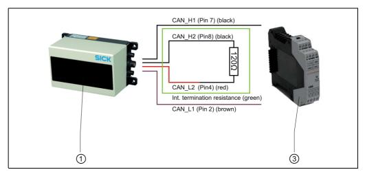
Fig. 5-7: Connect one CAN module to the CAN interface of the LD-MRS
