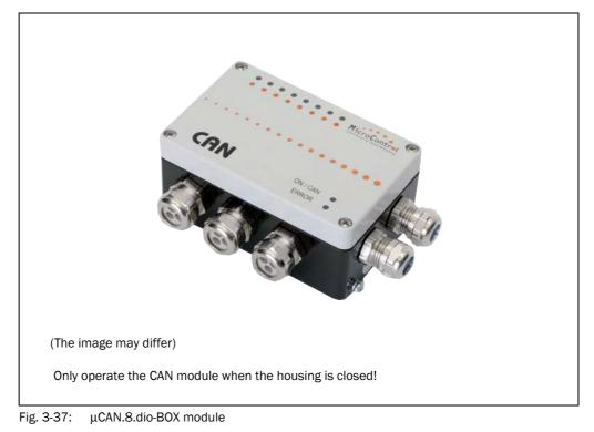
The address range of 1 to 127 is available in the CAN bus. By default, the LD-MRS has the address 1. The transmission rate of 500 kBit/s is fixed by the LD-MRS and needs to be set for the two CAN modules.
