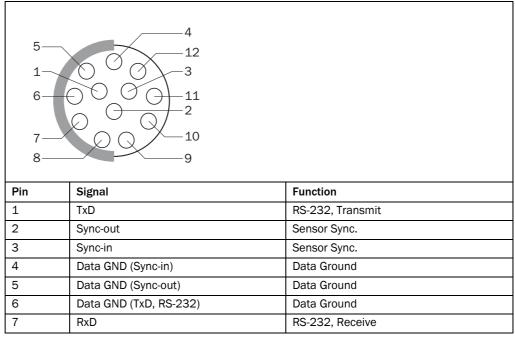
Tab. 5-2: Pin assignment of the 12-pin plug "data interfaces/synchronization" (round plug-in connection)
