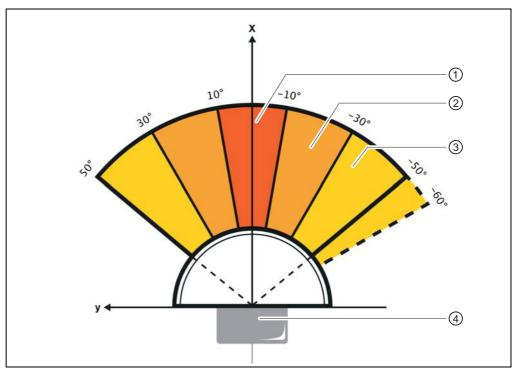
Fig. 3-12: Different angular resolution by sector
