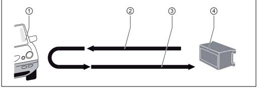
Fig. 3-2: Principle of time-of-flight measurement
