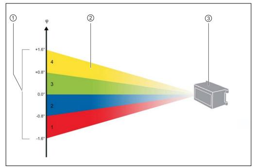
Fig. 3-5: Principle of the scan planes, color-coded
