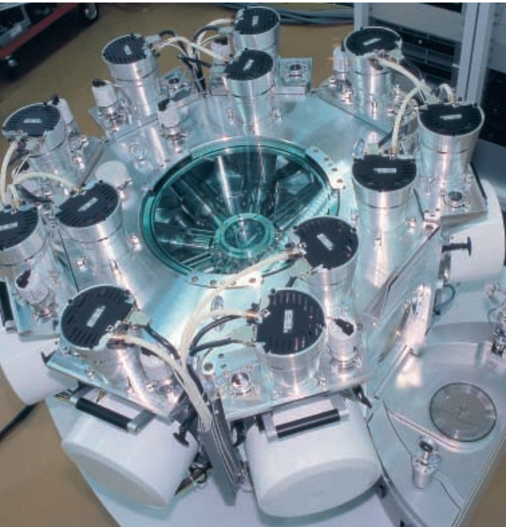
DVD Sprinter 8/8 from above: a look at the star-shaped transport unit which passes the disk from vacuum chamber to vacuum chamber
