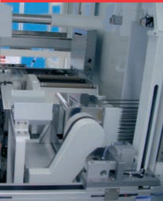
Wafer transfer from transport cassettes (FOUP) to the process carrier
