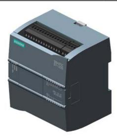
SIMATIC S7-1200, CPU 1211C, COMPACT CPU, DC/DC/DC, ONBOARD I/O: 6 DI 24V DC; 4 DO 24 V DC; 2 AI 0 - 10V DC, POWER SUPPLY: DC 20.4 - 28.8 V DC, PROGRAM/DATA MEMORY: 30 KB
