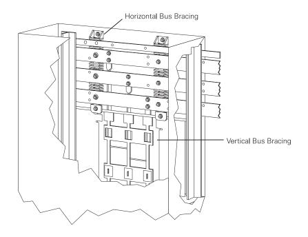
In addition, *NEC*<sup>®</sup> Table 430.97 requires 1" of clearance between a live bus and ground, 1" of clearance between phases through air, and 2" of clearance across a surface for voltages over 250 volts. These spacings are used throughout the horizontal and vertical bus in the MCC.
