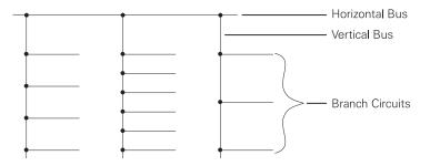
In power circuits, such as motor control centers, a bus is made of a heavy-duty metal bar. These bars provide power to each of the combination motor control units. The vertical bus is connected to a corresponding horizontal bus and is isolated from the other bus bars.
