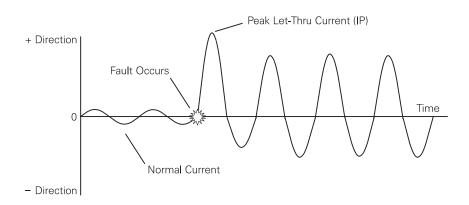
There is also energy let-thru  $(|^2t)$ . This destructive thermal force is capable of melting conductors.
