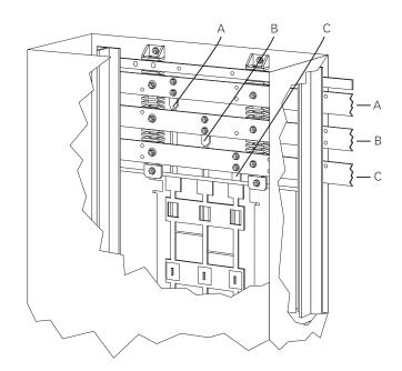
It should be noted that the NEMA phase arrangement illustrated in the previous drawing is viewed from the front. The vertical bus bars appear to be in reverse order when viewed from the rear. Some motor control centers can have devices installed on the front and rear of the motor control center.
