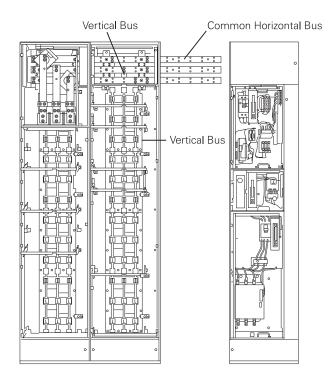
When there are more than four sections or the customer specifies a split between two vertical sections a splice kit between the horizontal bus bars can be installed.
