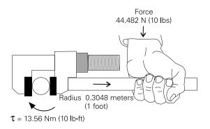
An increase in force or radius would result in a corresponding increase in torque. Increasing the radius to 0.6096 meters (2 feet), for example, results in 27.12 Nm (20 lb-ft) of torque.
