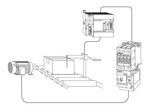
Another application might involve the use of an AC drive, such as a Siemens MICROMASTER, MIDIMASTER, or MASTERDRIVE. In this example a PLC is used to control a trimming cycle for a continuous roll. A sensor, connected to a PLC input, is used to detect a reference mark on the roll. An AC drive, controlled by the PLC, is used to control the acceleration, deceleration, and speed of an AC motor.
