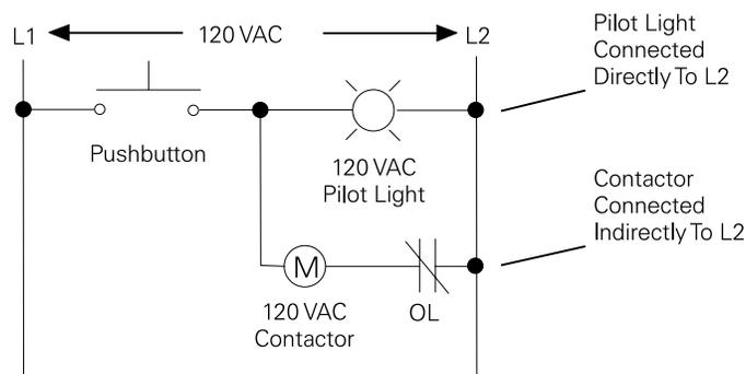
Control loads are generally not connected in series. The following illustration shows two ways to connect a control load. In one instance the control loads are improperly connected in series. When the pushbutton is depressed, the voltage across L1 and L2 is divided across both loads, the result being that neither load will receive the full 120 volts necessary for proper operation. If one load fails in this configuration, the entire circuit is rendered useless.
