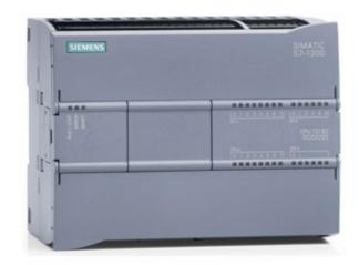
SIMATIC S7-1200, CPU 1215C, COMPACT CPU, DC/DC/RELAY, 2 PROFINET PORT, ONBOARD I/O: 14 DI 24V DC; 10 DO RELAY 2A, 2 AI 0-10V DC, 2 AO 0-20MA DC, POWER SUPPLY: DC 20,4 -28,8 V DC, PROGRAM/DATA MEMORY: 100 KB
